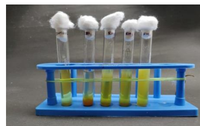
Fig.2 Ammonia production by the Rhizobium isolates in the presence of glyphosate herbicide
